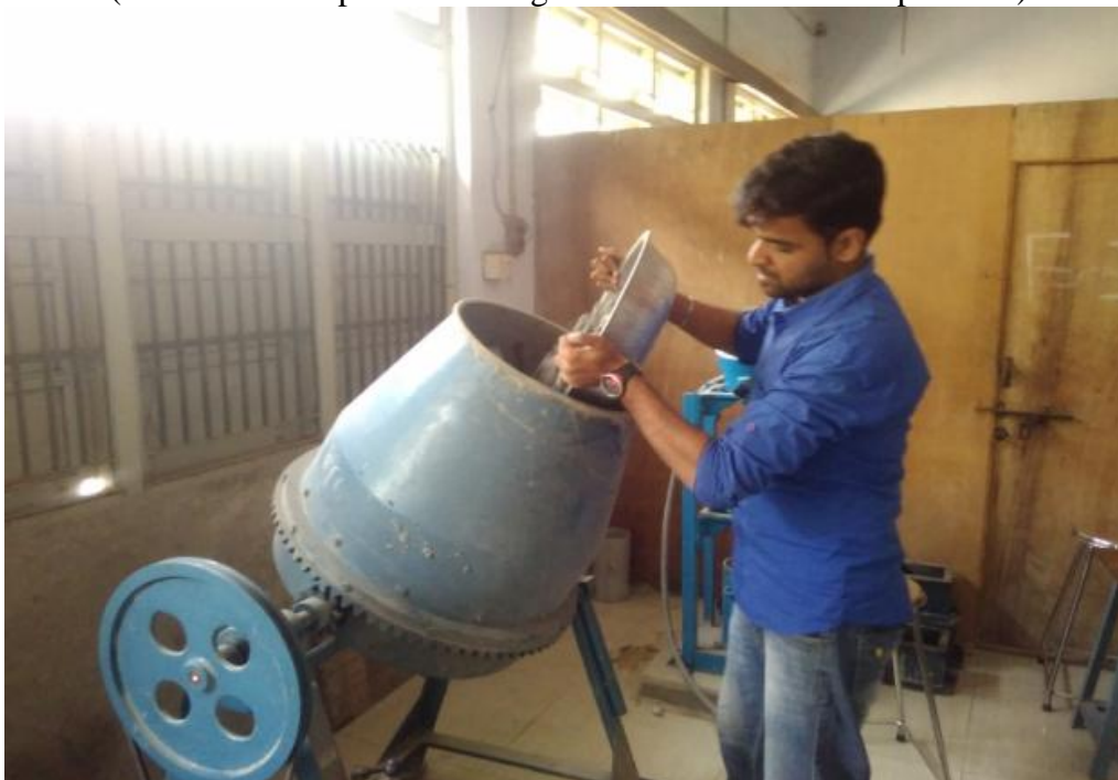
(Photo 4:- Mixing ingredients for the concrete)
