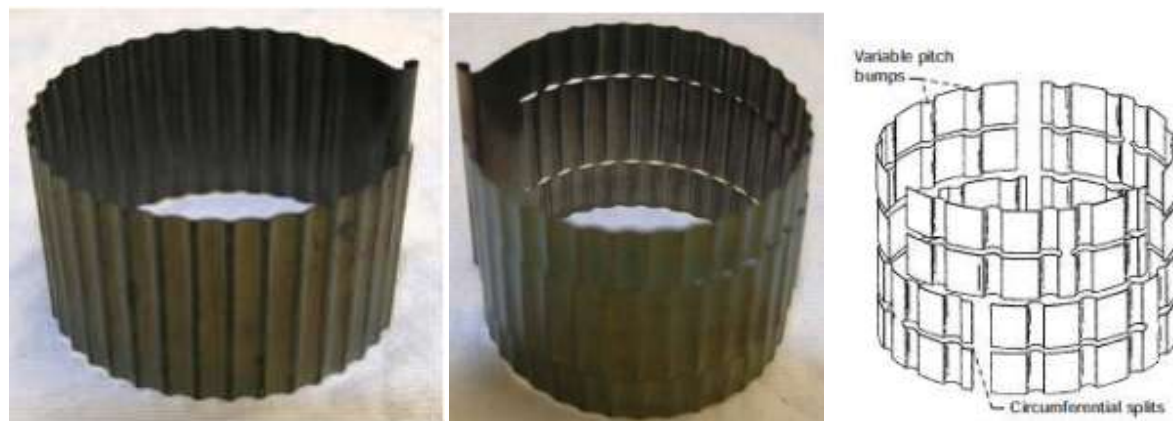
(a). Gen-I Bearing Foil (b). Gen-II Bearing Foil (c). Gen-III Bearing Foil Figure 9 Variation in foil structure in all three generation bearings [14]
