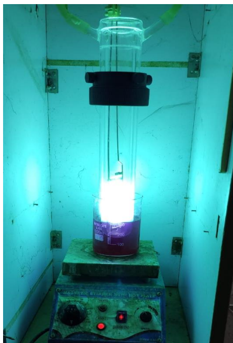
Figure 3. Photoreactor with 250 W Xenon UV-Vis lamp for degradation of fuchsin basic dye
