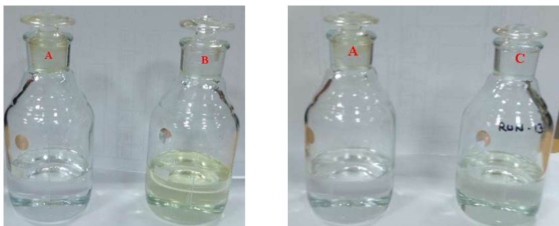
Fig.2. UV stability test (A) Untreated fresh base oil (B) Untreated base oil under 8 hour sunlight exposure (C) Hydro-treated base oil under 8 hour sunlight exposure
