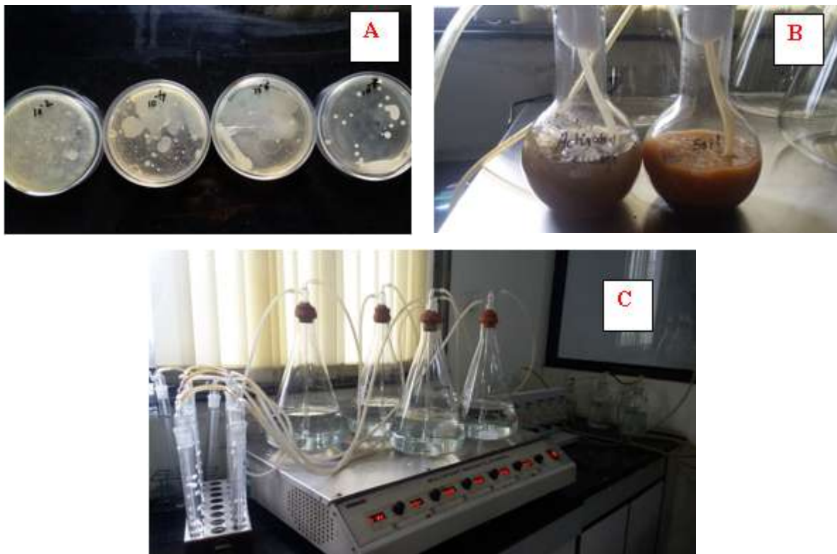
Fig.3. Sample preparation and test setup (A) Microbial enumeration (B) Activated sludge and moist soil sample in blender and aerator (C) OECD test setup
