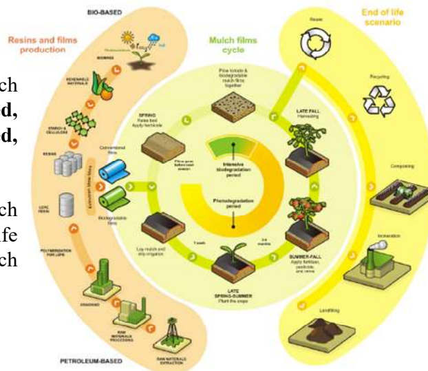
Figure 3. Cradle to gate, grave, and cradle life cycle flowchart of plastic mulch films. After removal of conventional mulch films, they can be reused, recycled, incinerated, and/or landfilled. Biodegradable mulch provides the same end-of-life scenario routes and also can be composted. [ref.18]
