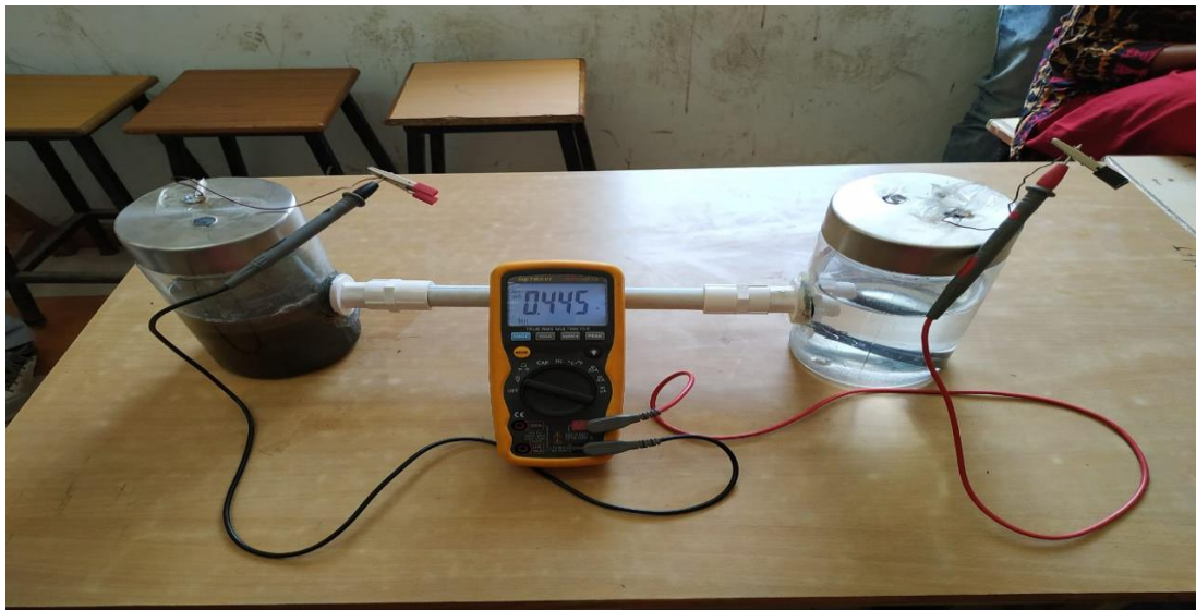
Figure 2. Photographic picture of the experimental MFC set up
